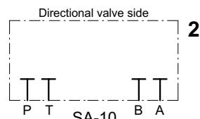
These blanking- or capping plates are used, for example, to blank-off spare subplate stations and can be used as the starting point for making special connection plates.
