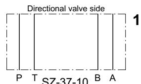
These plates are included as required to provide a simple spacer function
